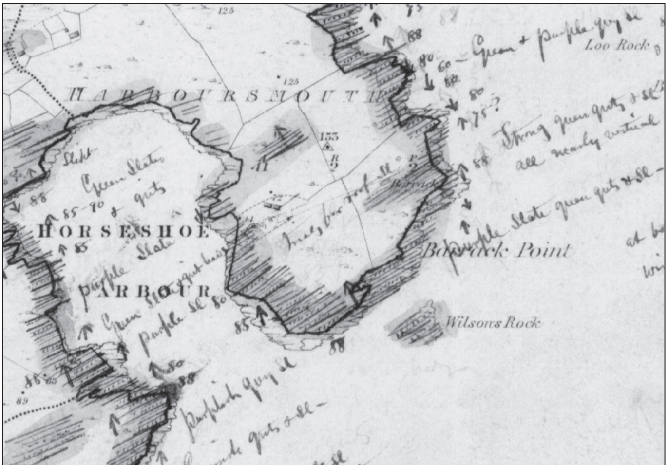
Figure 2. Geological Survey of Ireland fieldsheet for the Horseshoe Harbour area noting the presence of ‘greenish grits and slate beds’. ‘Quarry for roof sl’ is recorded adjacent to the quarry site
