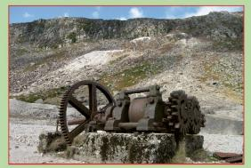
e Cornish rolls crusher at the early twentieth century White Rock treatment plant. Glendalough, manufactured by John Mills of the Railway Foundry, Llanidloes, Wales. This is the finest crusher of its type in Ireland and is of superlative heritaev sulue. See name to Sharron Schwartz and Murin Critichiev inside
