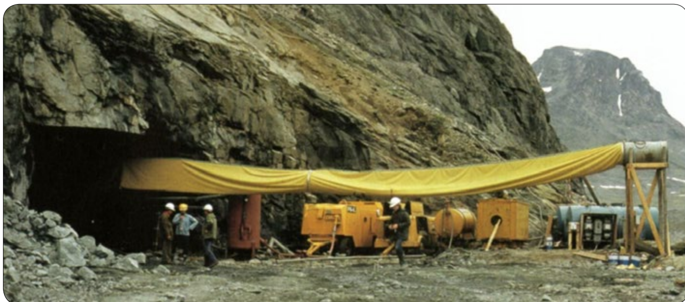
The entrance to the Kvanefjeld Adit in 1979. Note the ventilation system which kept the level of radioactive emanation at a very low level in the workings. The adit is now sealed to prevent people accessing the workings and being exposed to harmful levels of radioactive air (Image courtesy of GEUS)
