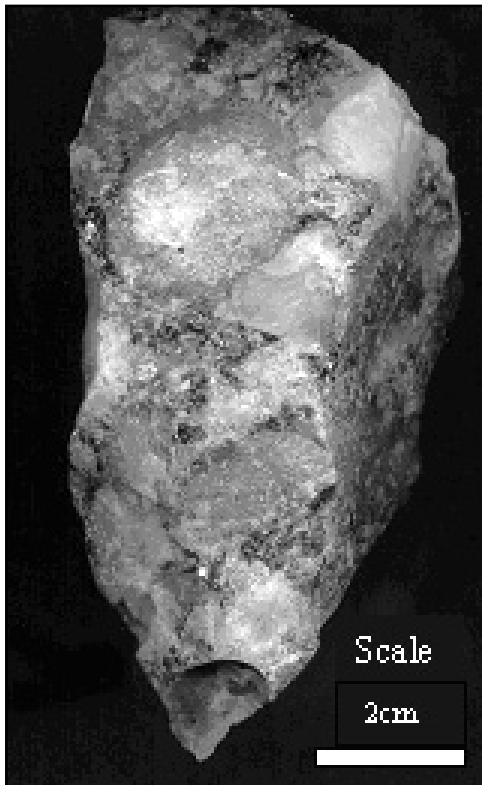
Figure 4. Keel ore showing zinc-blende (ZnS, sphalerite) as the darker patches, in the interstices of a pebble conglomerate.
