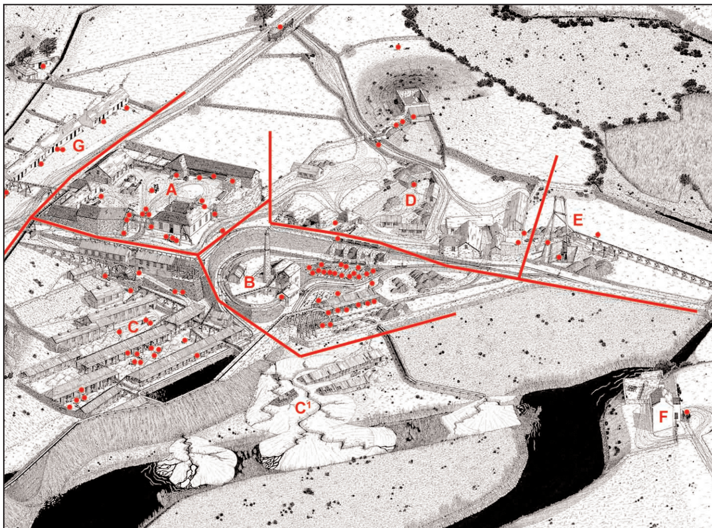
Figure 19. The ore dressing floors at Knockmahon as they might have appeared in about 1860: count-house yard (A); breaking, crushing and jiggling area, including engine-house and boiler-house (B); main dressing floor (C) including several sheds housing circular buddles (some sheds are shown ruined and disused on the valley floor, partially covered with mine waste: C1); gunpowder overlooking yards and sheds on different levels (D); Downright Shaft (E); mine manager's house (F); miners' cottages (G and G1). The red spots mark the locations of all the 93 people included in the reconstruction drawing.
