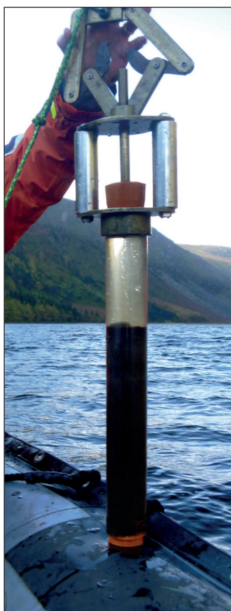
Fig. 4: GDL core after collection via modified Kajak-Brinkhurst corer
